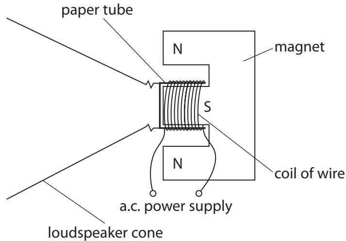
A coil of wire is wrapped around a paper tube attached to the loudspeaker cone.
